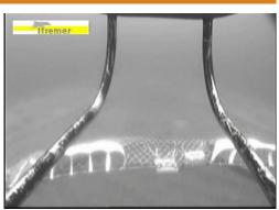
This flexible kite (made in canvas coated with PVC) can be used with bottom or midwater trawls.
