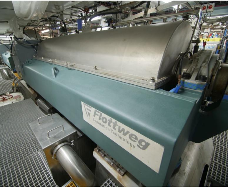
Onboard Starbound, the Flottweg equipment is used to separate the meat from the liquid.
